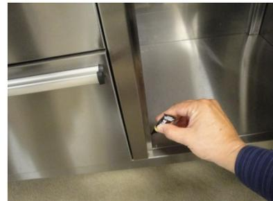
2. Assemble the black neoprene strip onto the door stopper. Starting at the bottom and with the straight edge of the strip facing downward, push the neoprene strip by hand onto the metal edge of the door stopper and work your way vertically until the entire edge is covered.
